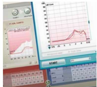
Real-ear measurement module - use On-Top mode to easily adjust the hearing instruments in real time during the measurement
