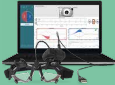
EyeSeeCam vHIT. A simple USB connected goggle and a laptop make this test easy to complete in any clinical setting.
