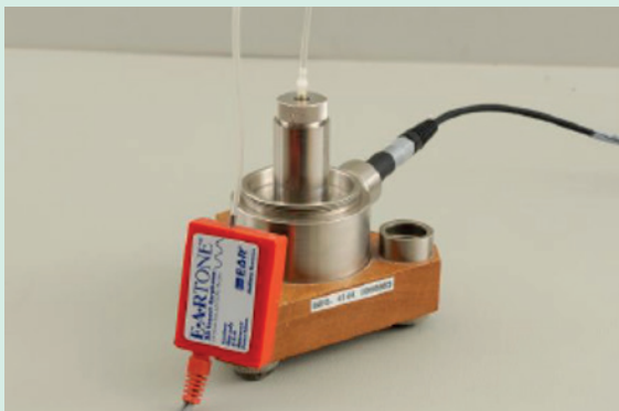
Figure 13 Calibration setup for insert headset on 2cc coupler with tube adapter.
