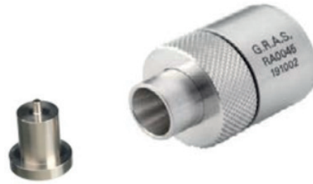
Figure 11 Ear simulator - often referred to as 711-coupler. Ear tip adapter is mounted; separate part is ear mold substitute with tube adapter.
