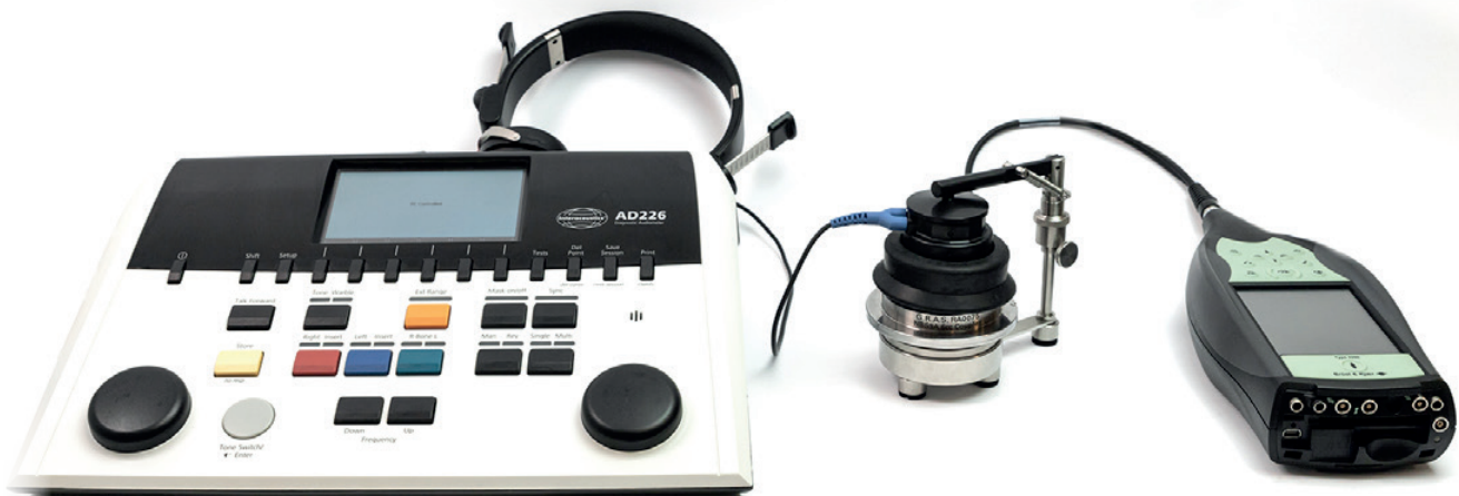
Figure 3 Typical setup for calibration equipment (transducer from audiometer is placed over coupler with microphone connected to sound level meter).
