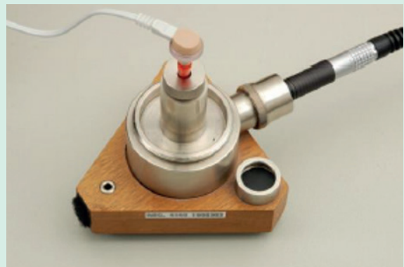
Figure 14 Calibration setup for CIR 22/33 on 2cc coupler with ear tip. Same setup is used for tympanometer probes.
