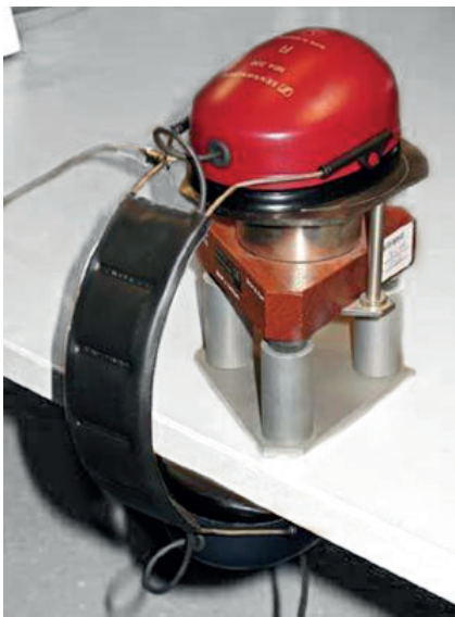
Figure 8 Calibration setup for Sennheiser HDA200 and Radioear DD450.
