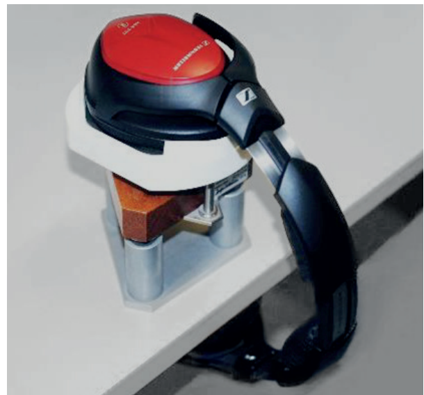
Figure 9 Calibration setup for Sennheiser HDA300 including mandatory centering adapter.
