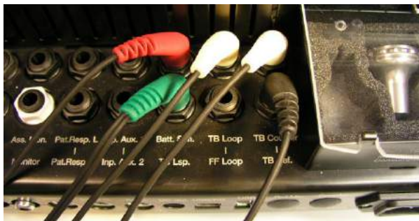
Figure 2: Cable placement on the Affinity/Equinox
