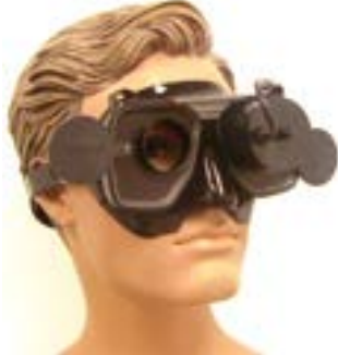
Figure 1.5-6 Placement of front mount camera in goggles
