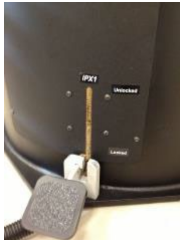
Figure 7.12-7 Foot brake applied
