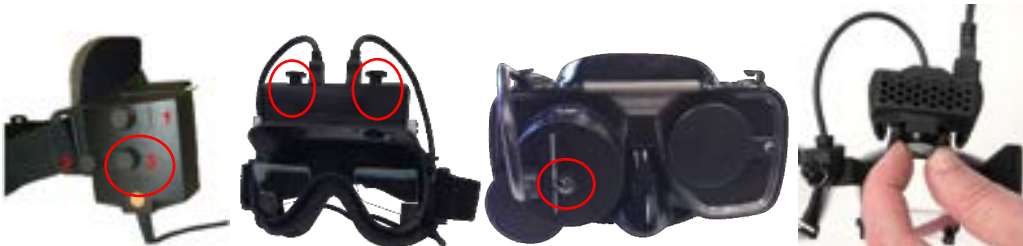
Figure 1.6-2 Adjustment control for focusing eye image on each camera
