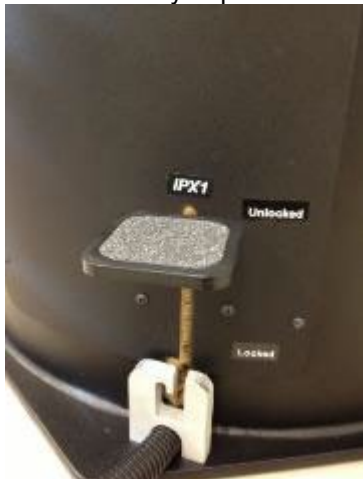
Figure 7.12-6 Foot brake released
