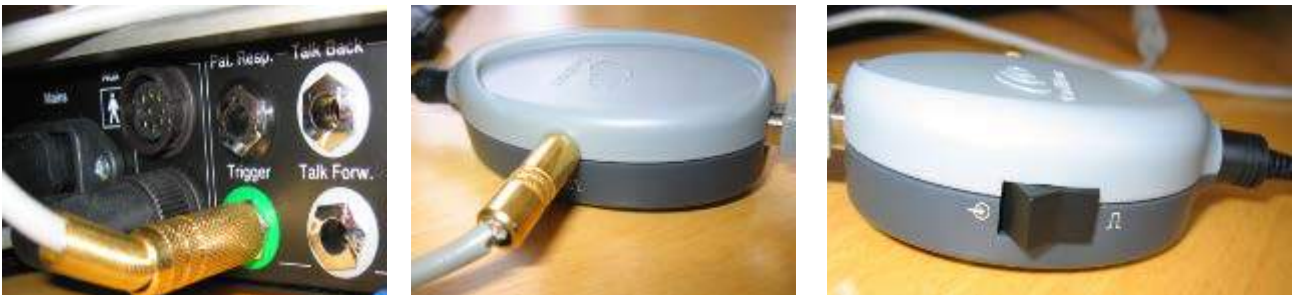
Left: The trigger socket on the back of the Eclipse. Center and right: The PPS box from Cochlear Nucleus and its setting.
