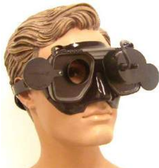
Figure 1.3.7 Placement of Front Mount Camera in Goggles
