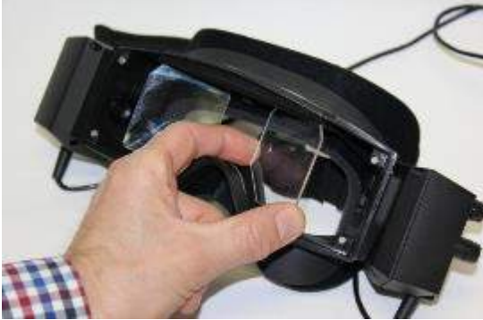
Figure 1.3.5 Mirror adjustment for smaller faces
