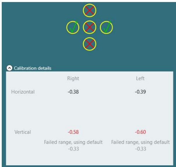
Figure 2.1.9 Calibration failure with values and failure reason
