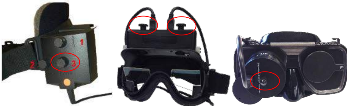
Figure 1.4.2 Adjustment control for focusing eye image on each camera
