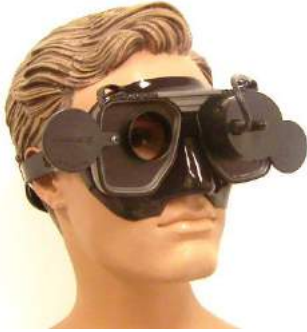
Figure 1.5-6 Placement of Front Mount Camera in Goggles
