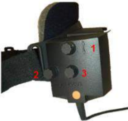
Figure 1.5-3 Side mount cameras adjustment knobs for regulating image and focus
