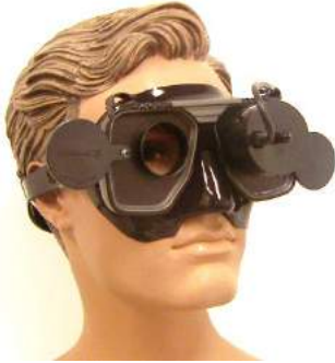
Figure 1. 5. 6 Placement of Front Mount Camera in Goggles
