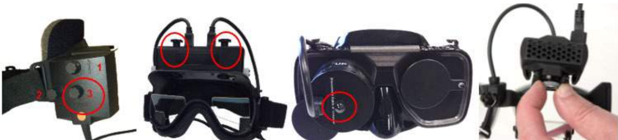
Figure 1. 6. 2 Adjustment control for focusing eye image on each camera
