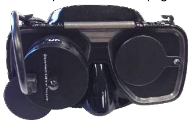
Figure 1. 16. 1 Front mount camera goggles with camera in right eye portal
