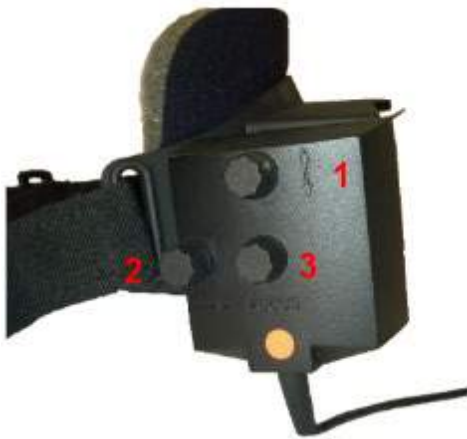
Figure 1. 5. 3 Adjustment knobs for side mount camera for regulating image and focus
