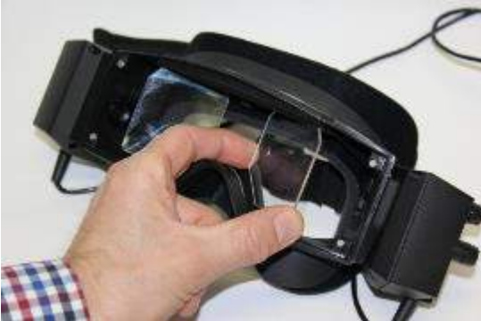
Figure 1. 5. 4 Mirror adjustment for smaller faces narrow inner canthal spaces
