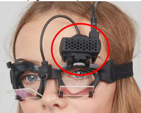
Figure 1. 5. 7 ESC cameras adjustment knobs for regulating image
