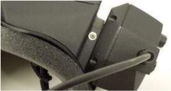
Figure 1. 16. 2 Side-mount camera goggles hex screw for attaching camera module
