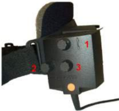
Figure 1.5-3 Side mount adjustment knobs for regulating image and focus
