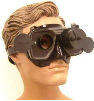
Figure 1.5-6 Placement of front mount camera in goggles
