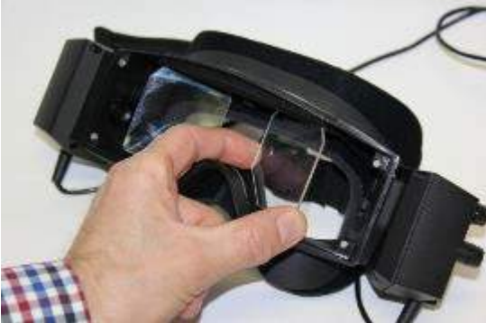
Figure 1.5-4 Mirror adjustment for smaller faces or narrow inner-canthal spaces
