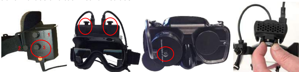
Figure 1.6-2 Adjustment control for focusing eye image on each camera
